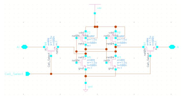
Writing data to the cell is accomplished by overpowering the internal transistors to "flip the bit." Only writing a low voltage (actually 0V) will work, because the NMOS pass gate passes a logic '0' better and the PMOS transistor is easier to overpower. Therefore, a low voltage on the "A" bitline writes a zero to the cell, and a low voltage on the "Ai" bitline writes a logic one into the cell.
