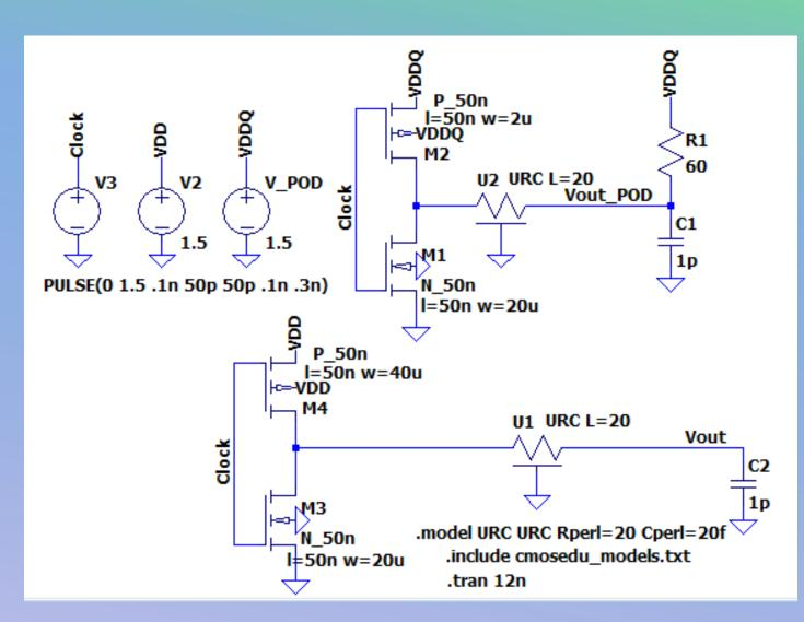
In this simulation we see that the output swing is slightly larger peak-to-peak for the push-pull driver, yet we finally have a smaller current draw (and thus power dissipation) for the POD driver.
