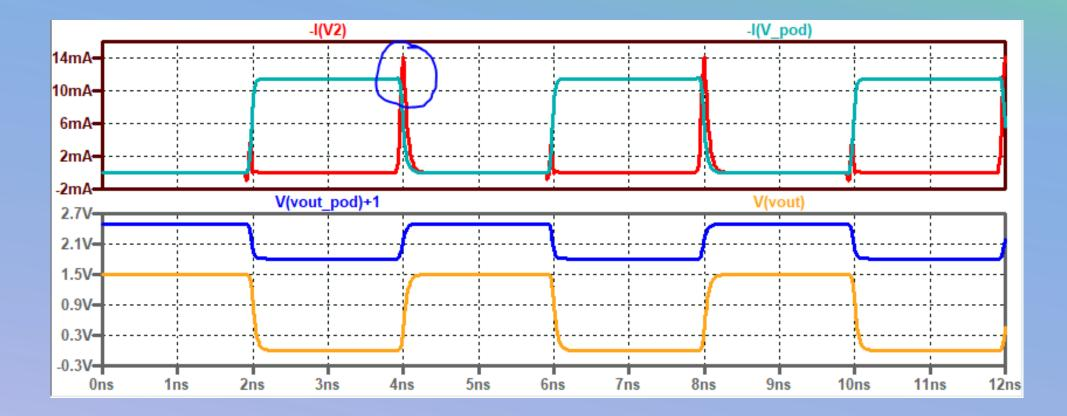
To simulate the high frequencies in a memory bus we increase the clock frequency and also increase the RC delay through the transmission line.
