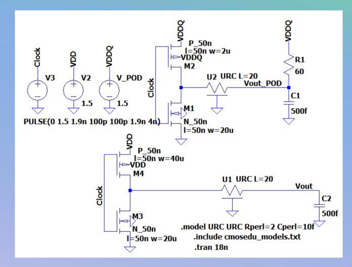
At the simulated low frequency (relative to delay of the transmission line) the static power draw of the POD driver dominates, but note the indicated current transients for V2 are significantly larger.
